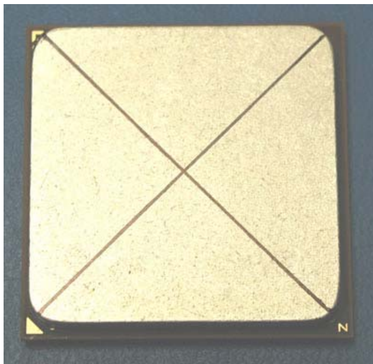
Figure 16. Diagonals Marked on Processor to Locate Center
